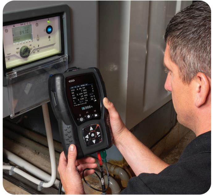
Testing boiler efficiency
