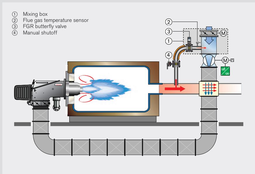
General arrangement of an FGR system with WK-series burner and mixing box in hot-air execution for flue gas temperatures  $\leq 300$  °C before the combustion air preheater.
