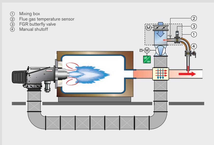
General arrangement of an FGR system with WK-series burner and mixing box in hot-air execution for flue gas temperatures  $> 300$  °C after the combustion air preheater.
