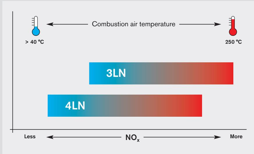
NOx behaviour on WK burners with preheated combustion air
