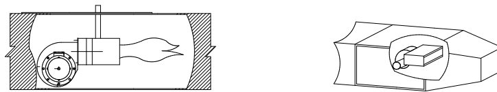
The SP arrangement includes an integral combustion fan and burner side-mounted inside the air duct.
