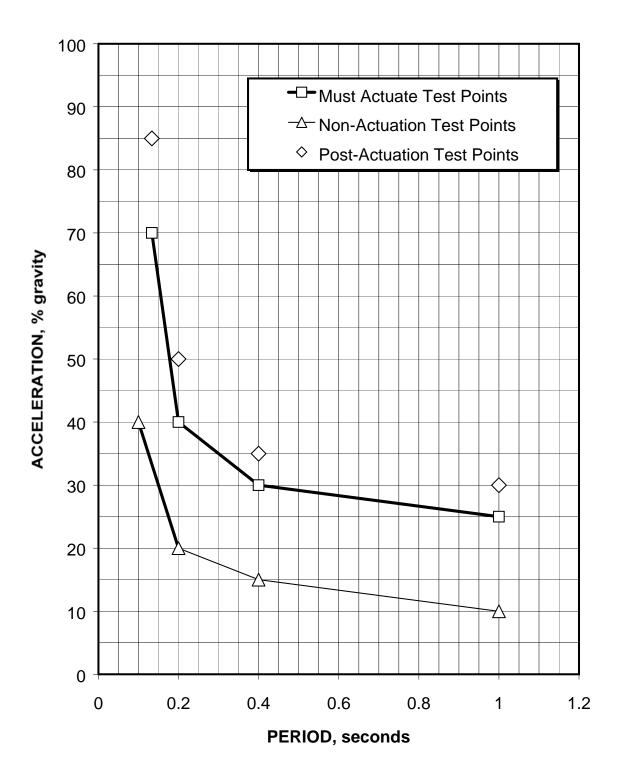
Actuation ranges of ASCE Standard 25-97 for Earthquake Actuated Automatic Gas Shutoff Devices
