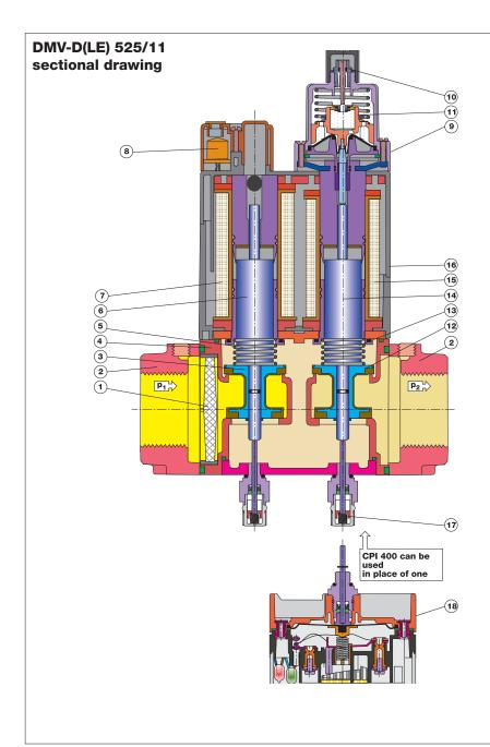
Strainer 1 2 Flange Valve V1 3 4 Housing 5 Closing spring V1 6 Plunger V1 7 Solenoid V1 8 Electrical connection 9 Max flow adjustment 10 Initial lift adjustment (DMV-DLE) Hydraulic brake (DMV-DLE) 11 Valve V2 12 Closing spring V2 13 14 Plunger V2 15 Solenoid V2 Solenoid housing 16 17 Visual indicator (VI) CPI 400 interlock switch 18
