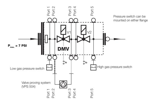
Position Indicator: CPI 400 interlock switch on V1 or V2, or on both Visual Indicator (VI) on V1 or V2, or on both
