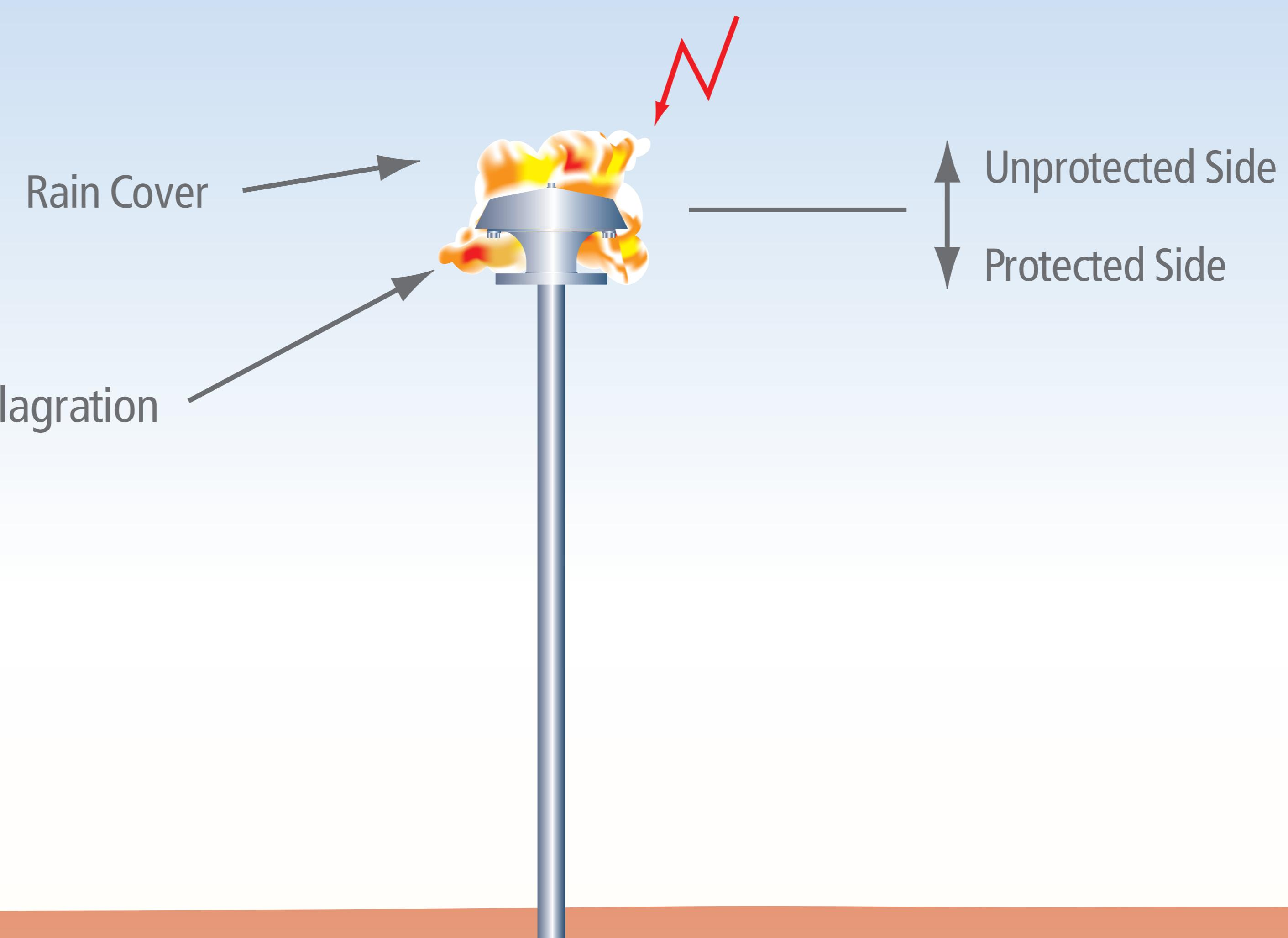
End of line deflagration flame arresters prevent an ignition in the surrounding atmosphere from entering the vent pipe.
