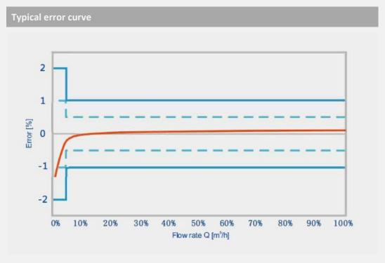
The rotary meters TYL show very stable and reproducible measurement results. The design of the housings and pressure containing parts has been optimized especially for robustness under torsional and bending stresses. The meters can withstand more than double the specified torsional and bending stresses implied through the installation as defined in EN 12480.
